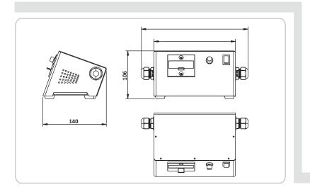
: TimiT 02. Model No Part Number : 20-14-0071. Input voltage : 230V AC, 50Hz.
